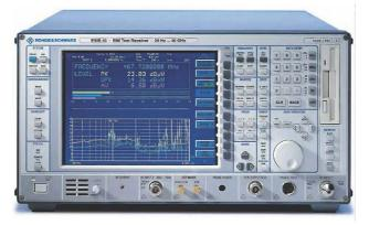
EMI (electromagnetic-interference) test receivers, such as this unit from Rohde and Schwarz, are among several specialized classes of instruments that play major roles in the testing of products that implement UWB.
