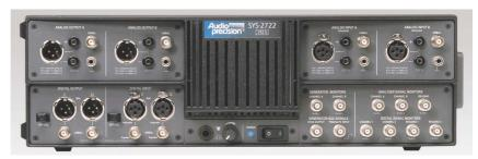
Figure 1 The Audio Precision SYS-2722 dual-domain audio analyzer drives and receives signals on balanced and unbalanced feeds in the analog domain and through balanced, unbalanced, and optical connections in the digital domain.
